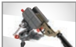
Optimally position lower receiver to install buffer and buffer detent pin.
