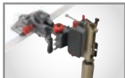
Position the barrel and upper receiver downward into the trash for bore and barrel cleaning.
